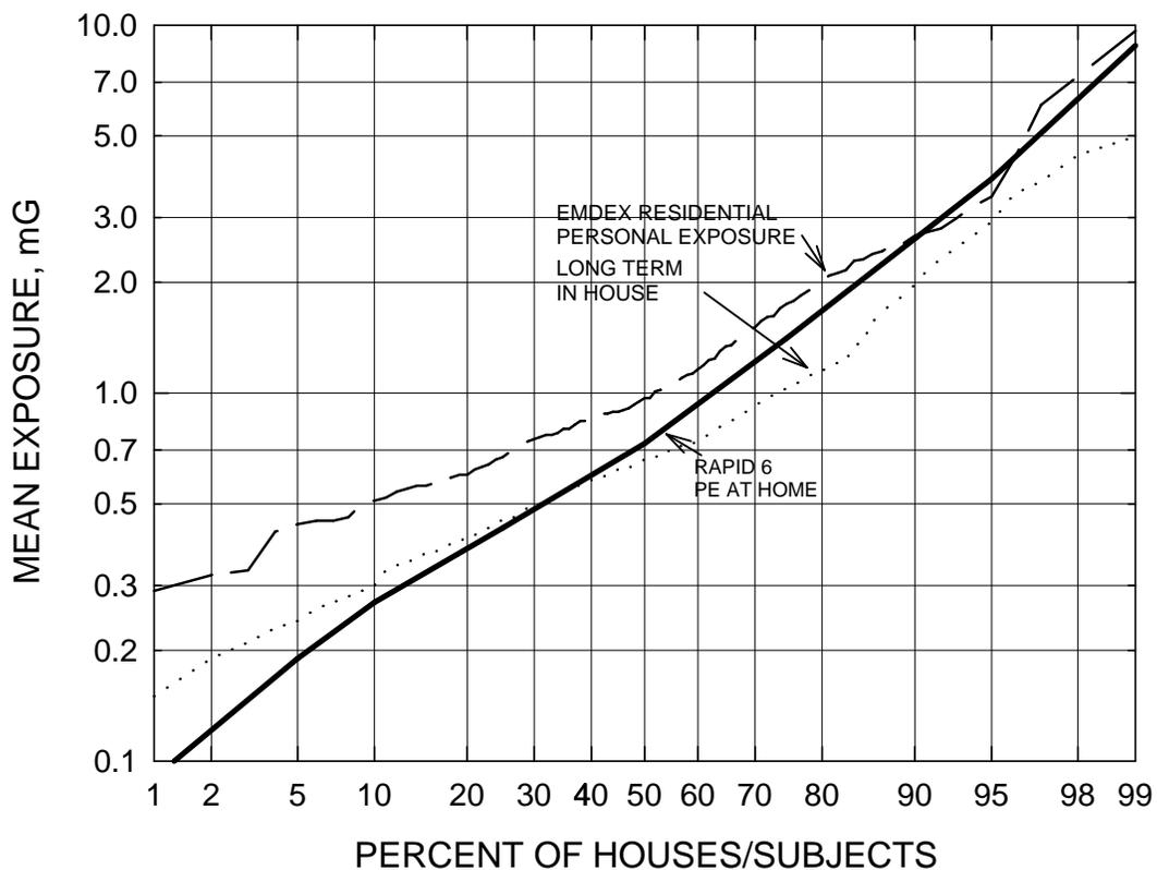
**Figure 12-1. Distributions of average long-term measurements from EMDEX Residential Study and of average at-home exposures while wearing PE meter for the EMDEX Residential Study and RAPID Project #6, respectively. (Bracken et al., 1994; Zaffanella and Kalton, 1998b)**
